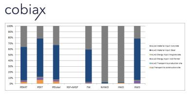
The impact indicators are also significantly influenced by the production process associated with the base materials concrete and steel (90-97%). In the case of ODP, POCP and ADPF in particular, the steel component is dominant for flexural reinforcement and hollow reinforcement cases.
