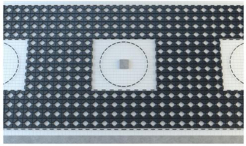
Cobiax installation modules are available for concrete slabs from 20 cm to over 80 cm. Roughly 50% to 80% of the floor area is laid with void formers, depending on the load and the static system.
